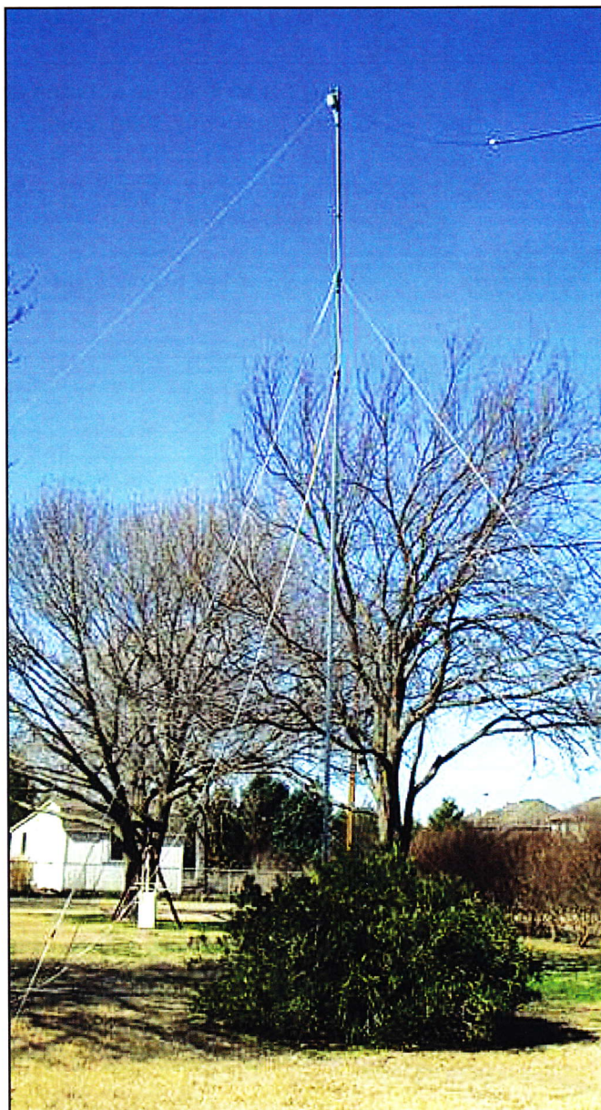
Photo A. The 40-, 20-, 15-, 10-meter off-center-fed antenna in an inverted-V configuration during testing. The apex height is 33 feet.
